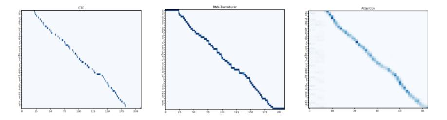
**Fig. 3**. Visualization of learned alignments for the same utterance using CTC (left), RNN-Transducer (middle), and Attention (right). The alignments are between ground-truth text (y-axis) and audio features fed into the decoder(x-axis). Note that Attention does two more time-scale downsampling, which results in  $4 \times$  shorter sequences (x axis) compared to the other two.
